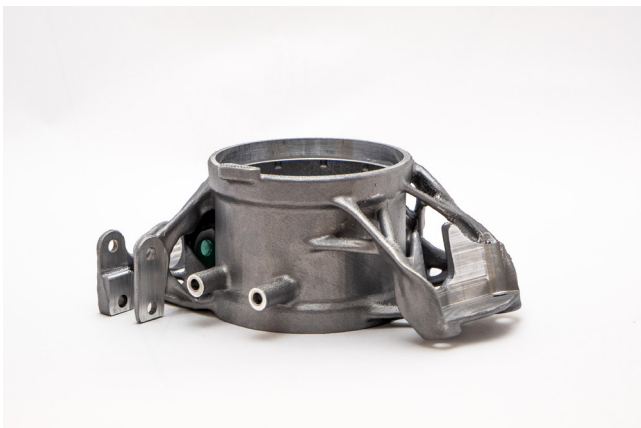
Optimized wheel carrier produced by 3D printing. Assembly process with suspension and brake system
